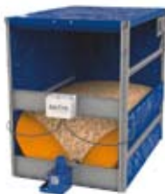
2. Now air cushions press the pellets against the auger.
